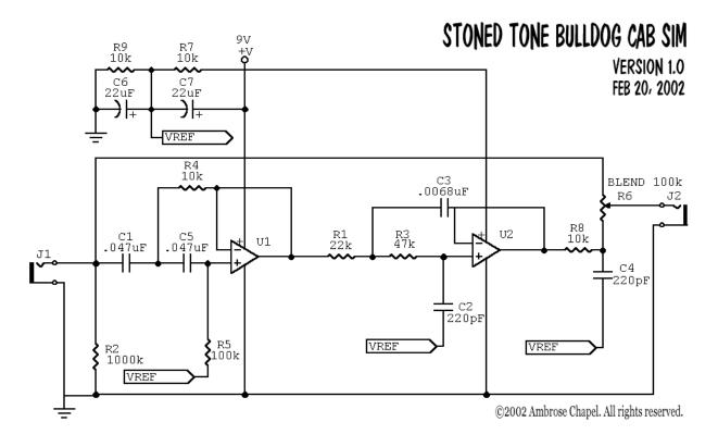
Bypass switching etc. isn't shown or needed depending on your application. Just one control "Blend". It blends between the straight signal and the cab sim. Here's a frequency plot to illustrate(Purple - Unaffected signal, Blue - Blend at 50%, Red - Fully affected):
